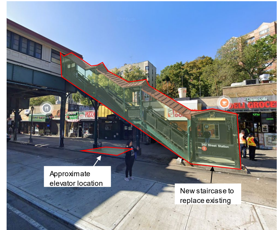
West staircase to be demolished and replaced with elevator headhouse and new staircase
